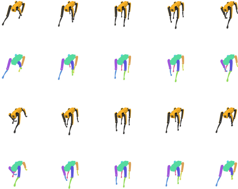
Figure 6: Manually defined walking animation for the Spot from the Robots dataset.
